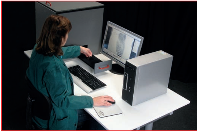
MUSCH SD150: Compact digital fingerprint evaluation workstation
